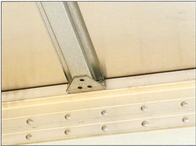
Roof bows are constructed of heavy-duty galvanized steel set on 24"/16"/24" centers with a one-piece roof skin for maximum strength and durability.
