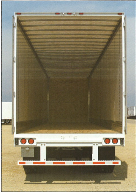
The Z-Plate® van has a full 110" inside height/rear door opening and 101" inside width scuff to scuff, and rear door opening for maximum payload. Taillights are recessed for maximum protection from damage. The reinforced rear bumper meets DOT requirements and is bolted on for easy repair if necessary. Rubber dock bumpers are standard.
