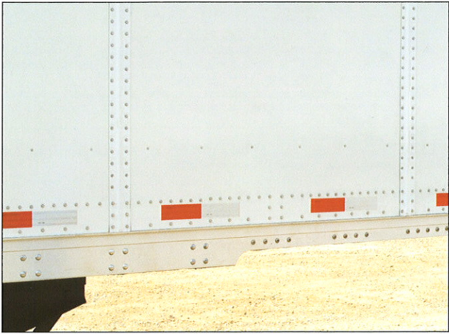
Exterior splice plates are coated with a tough baked on epoxy finish to match the exterior panel walls. Splice plates are riveted to composite panels 1 1/2" on center for added strength and durability.
