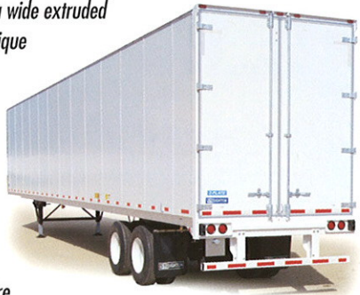
Front and rear top mounted clearance lights and rear ID lights are LED.
