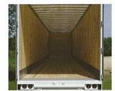
Standard 98" x 109-7/8" rear door opening allows easy access with an inside capacity of 3577 cubic feet for a 48' trailer and 3953 cubic feet for a 53' model.
