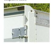
Built-in reinforcements in rear frame provide extra strength to help prevent racking without sacrificing inside door clearance.
