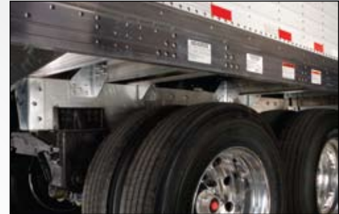
The suspension subframe is available in aluminum with galvanized steel gussets or undercoated steel.
