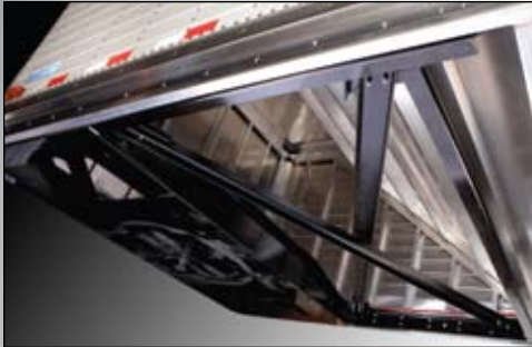
King Pins is set at 20". Cross bracing is 4" channel. Vents are available front & rear.
