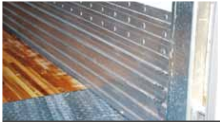
ULTRAPLATE XD Heavy duty bottom rail 16" high kick plate and 1/2" thick rib
