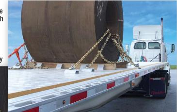
The trailer floor features an integrated load securement system to improve safety and convenience. The patent pending design is made possible by 3D solid modeling, FEA and friction-stir welding technology. The genius of the system is its simplicity. Modular chain tie-downs slide in grooves that are built into the floor. You can position the tie-downs virtually anywhere on the deck to secure your loads faster and easier with improved safety.
