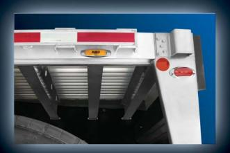
THREE STEEL CROSSMEMBERS PROVIDE ADDED STRUCTURAL SUPPORT AT THE REAR OF THE TRAILER TO HANDLE THE PUNISHING CONDITIONS ASSOCIATED WITH LOADING AND UNLOADING
