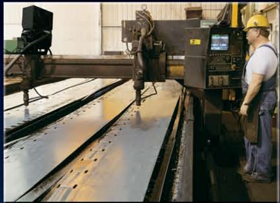
Computer controlled cutting assures the dimensional integrity of the Fontaine XtremeBeam®.
