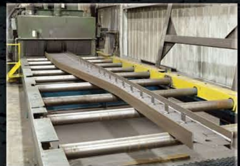
Paint adhesion is dramatically improved by an automated cleaning process.
