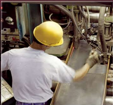
Robotic welding on both sides of the 3/8" x 5" top and bottom flange provides greater strength.
